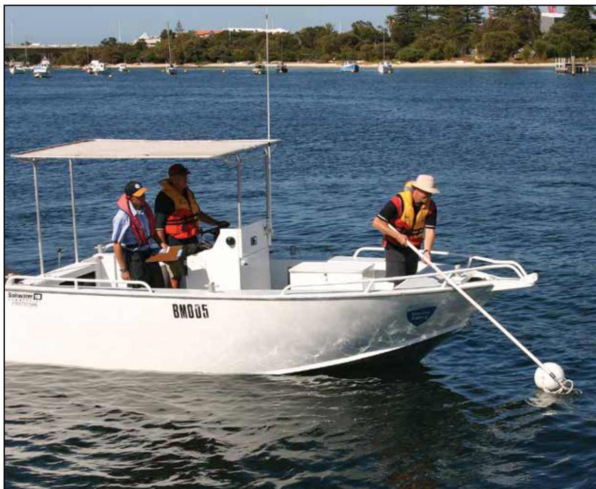
Turn the engine off before retrieving MOB
