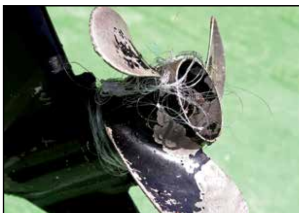
Check the propeller regularly for dents and damage and the shaft for snagged fishing line.
