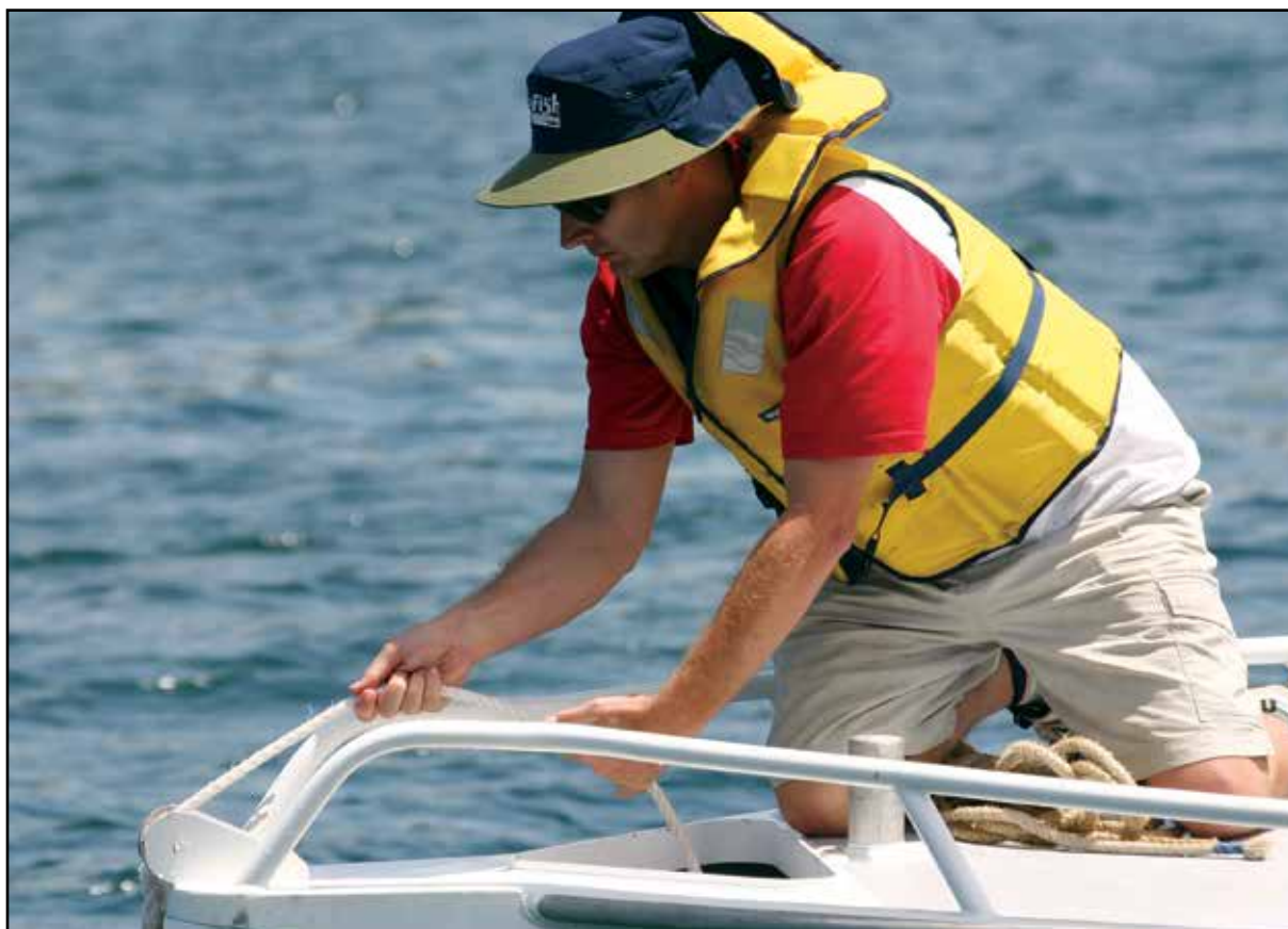
Anchor cable should be coiled neatly when retrieved so that it can be ready for instant use.
