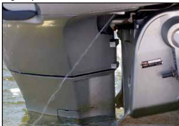
Check the telltale to be sure it is working.
