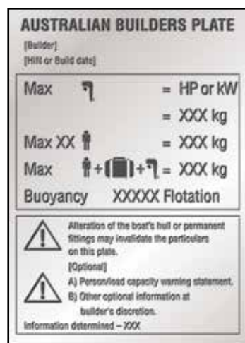
The Builder's Plate is compulsory for all vessels built after mid 2006.
