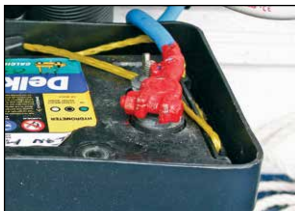
Check battery terminals for dirt and corrosion.
