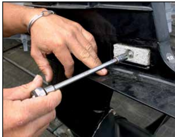
Check anodes for erosion.
