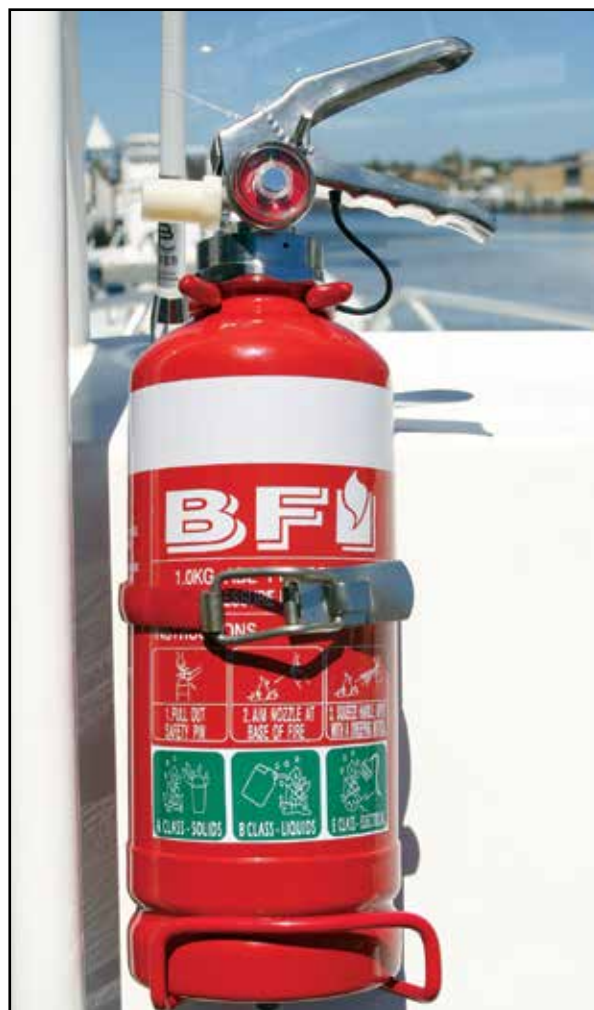
Fire extinguishers should be mounted securely and in an accessible location.
