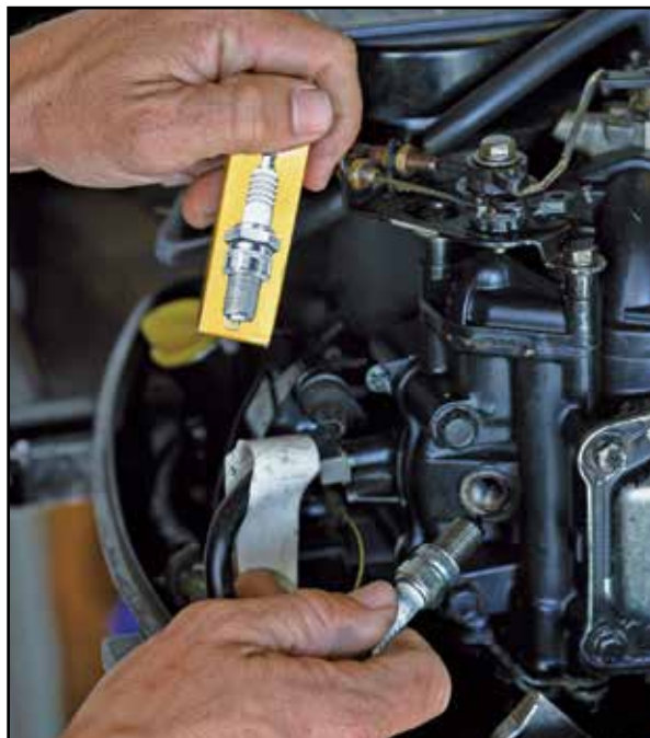
Carry a spare set of new plugs and a plug spanner.
