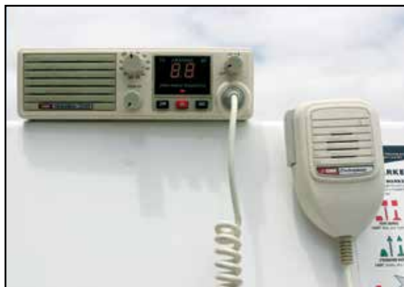
27 MHz radios and operators do not require a licence.
