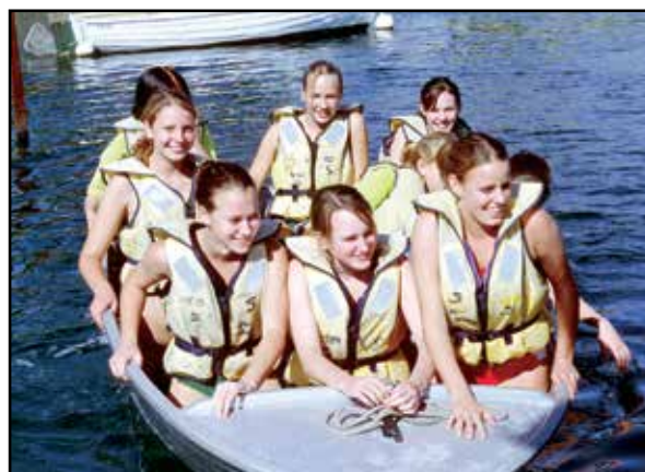
Overloading can seriously affect the vessel's stability.
