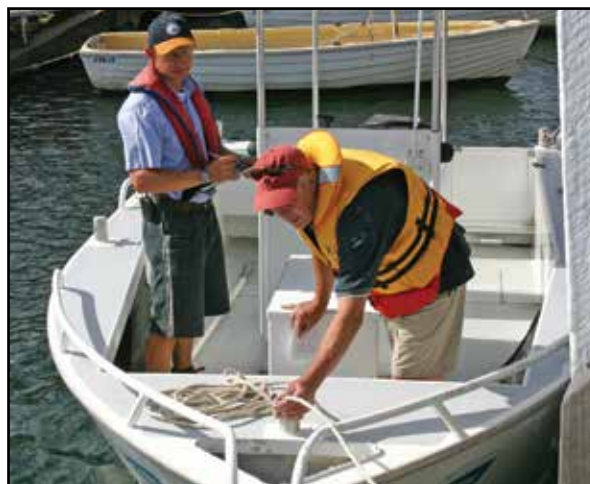
Check that lines are in a good condition.
