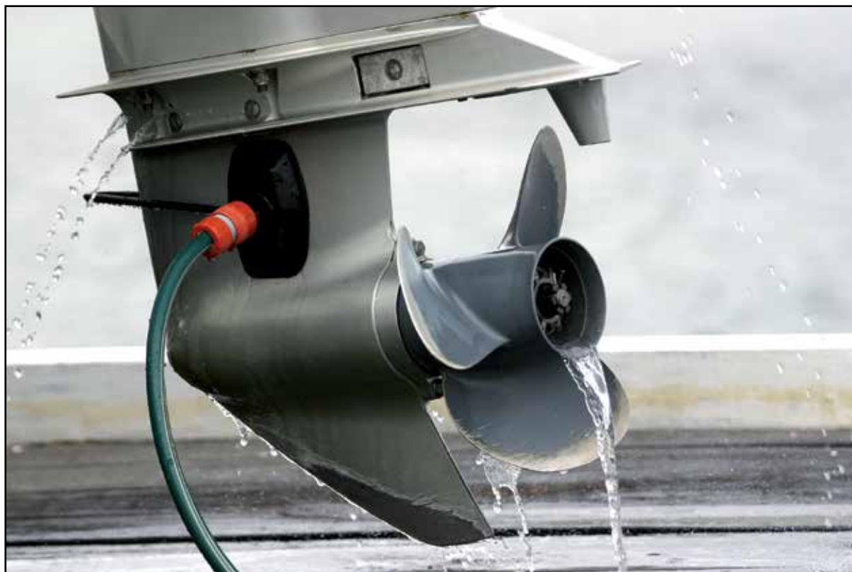
Flush the motor and wash it down with fresh water after each trip.
